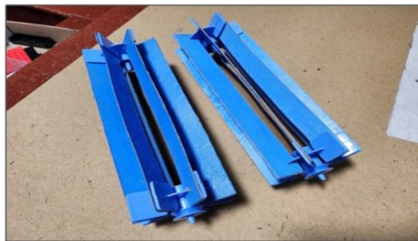
Figure 6. 3D printed horizontal turbine.
