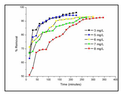
Figure 3. Removal of various initial copper ion concentration variations with time
