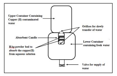
Figure 1. Experimental set up for removal of Copper (II) ion from aqueous solution
