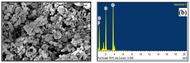
Figure 2. (a) FESEM image of HAp powder (b) EDX of Hap
