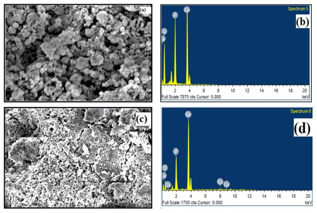
**Figure 4.** (a) FESEM image of HAP before adsorption, (b) EDX analysis of HAP before adsorption, (c) FESEM image of HAP after adsorption, and (d) EDX analysis of HAP after adsorption
